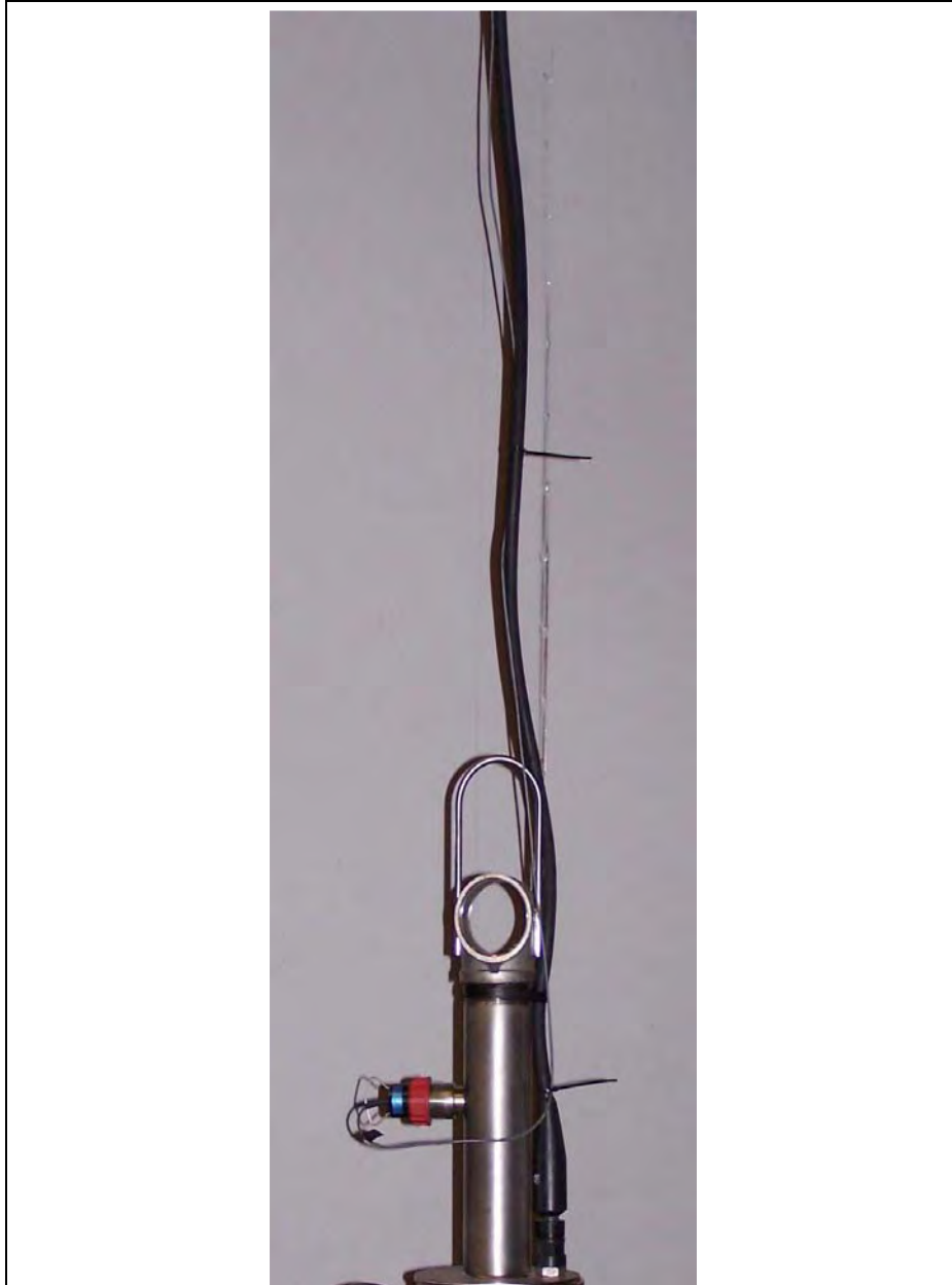
Figure 4.1.6 PSC-100P Power Cable zip tied to the FM-100 flow sensor cable PP-260SC shown, PP-100SC pump similar.
