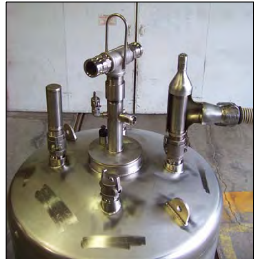
UD-36A with SHCK installed (above) on right vessel inlet. Left vessel inlet has the standard inlet safety screen installed.
