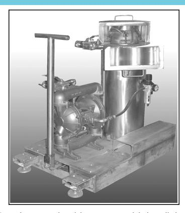
In nuclear power plants it is necessary to minimize radiation levels by periodically cleaning out settled sludge from sumps,
