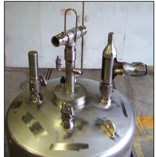
UD-36A with SHCK installed (above) on right vessel inlet. Left vessel inlet has the standard inlet safety screen installed. UD-48 Similar.
