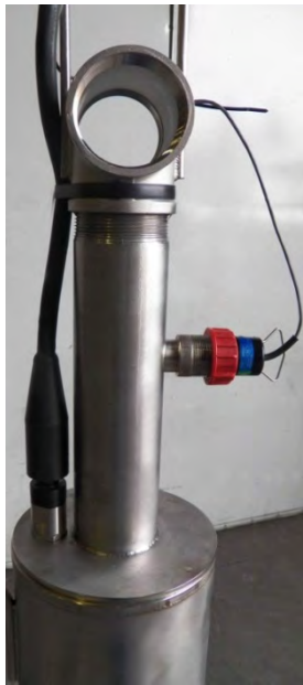
Figure 2.2 PP-260SC pump cover installed in a UFV-260 Housing UD-48A similar
