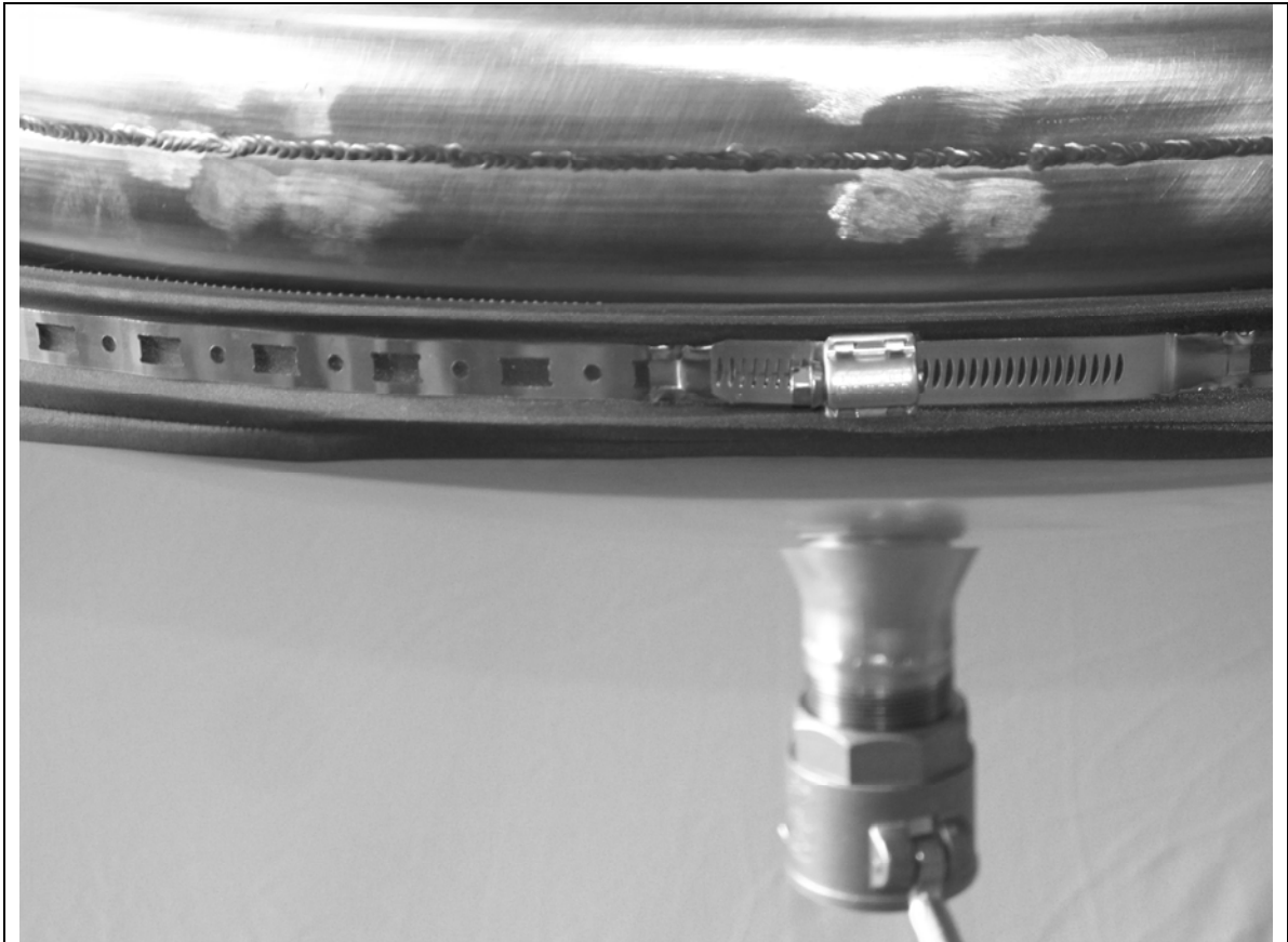
Figure 5.3 – SK-175 with the Skimmer Skirt band installed
