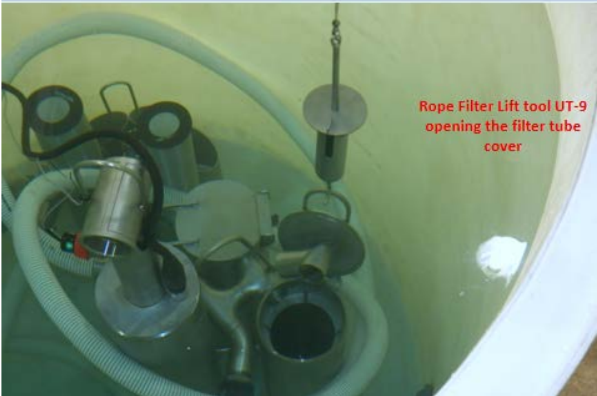
Rope Filter Lift tool UT-9 retrieving a filter to install in the UFV-260
