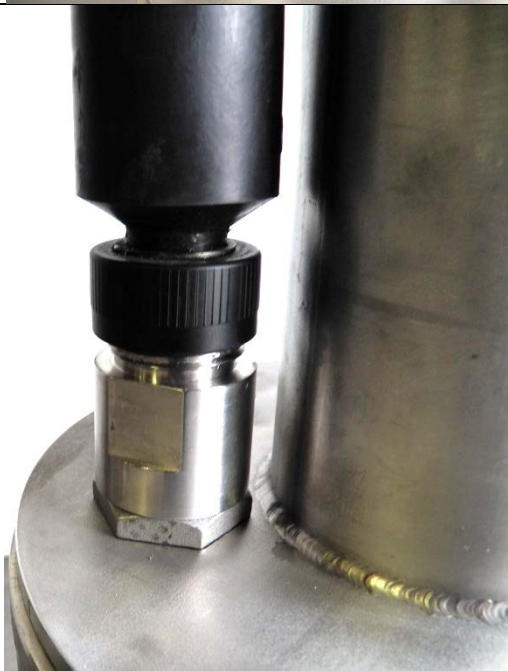
Figure 4.1.6.1 PSC-100P being installed on a PP-xxx-SC pump
