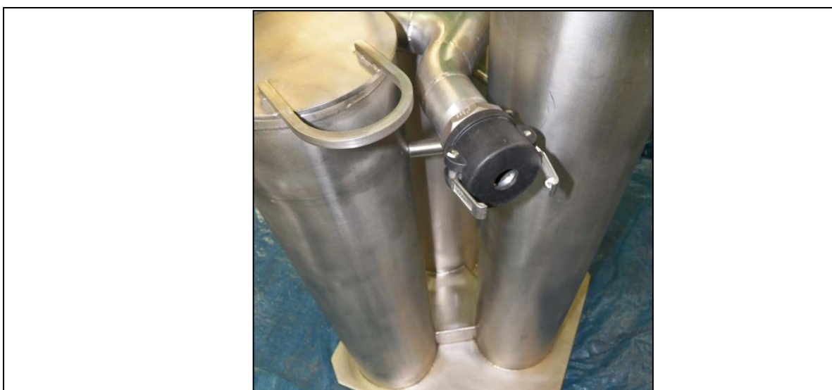
Figure 4.2.2.2 UT-12 Orifice Cap installed on the UFV-260 Housing
