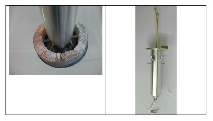
As the top pull rod is operated up or down in the tool housing, the hinged arms rotating on an internal cam will extend either in or out through the two open slots. The hinged arms will capture the filter for lifting, or release it for withdrawal of the tool.
