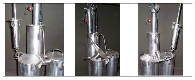
3.5 Next, lower the tool down into the open top of the expended filter cartridge until the top plate of the Rope Filter Lift Tool seats on the top of the filter cartridge. This is determined by a sudden decrease in the weight of the tool on the UT-15, Stainless Steel Utility Chain or nylon line.
