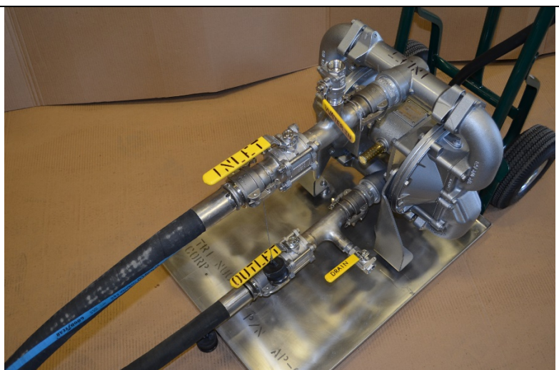
Hoses attached to the AP-65 with the inlet and outlet valves open
