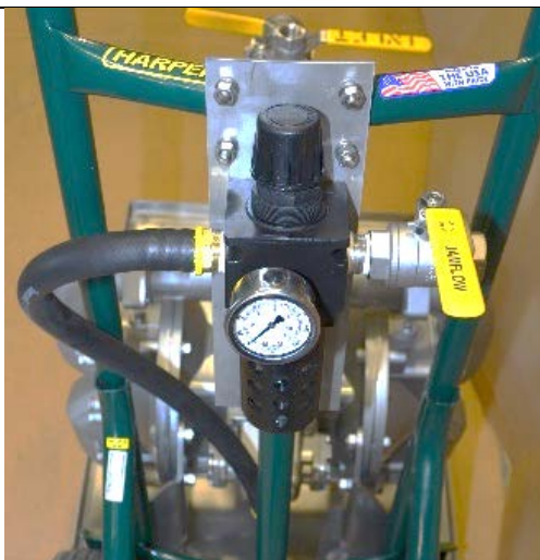
Air regulator and isolation valve on the AP-65
